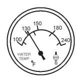
Figure 49. Coolant Temperature Gauge
